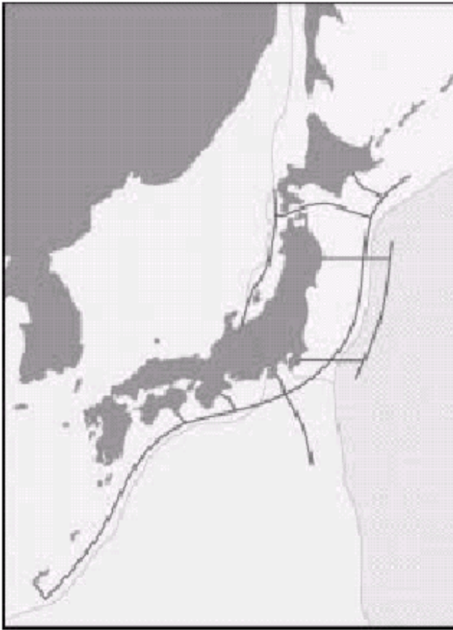
Fig. 7 Future cable network of ARENA
